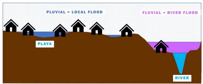
FIGURE 2-5 VISUAL REPRESENTATION OF PLUVIAL AND FLUVIAL FLOODING
